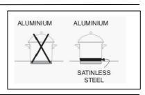
Hotplates should not be switched on without a pan on top. The base of the pan should be flat and dry. Pans that have been used on gas cookers are not normally completely flat and absorb heat badly.
