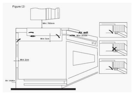
For safety the gap between the hob and any cupboard above it should be at least 760mm.
