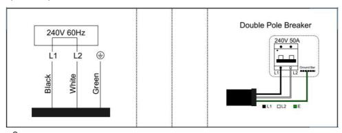
Black live wire L1, white neutral wire L2, green ground wire. The whole machine cannot be powered on if any of the black and white wires are not contacted well.
