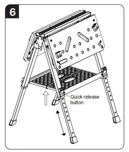
According to the arrow on the picture, it is convenient to quickly fold and shrink the leg
