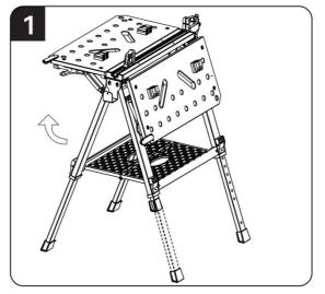
**NOTE:** Before using, check that the table is horizontal To use as a work bench, press leg button to extend the legs to the top position fully open the legs and pull the table top upward to make a work surface.
