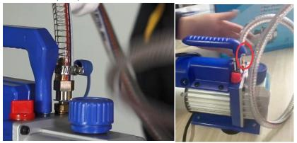
3. The interface at the other end of the hose is connected with the vacuum gauge, and the valve switch is shown in the figure.
