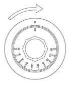
1. After installing the product, the temperature control switch knob is in the position shown in the picture, ready for work.
