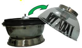
Remove the top from the flower trimmer's base. The inside of the top contains the high-density rubber tongues that are used to push the plant leaves into the blade grill. The cutting blades or wires are located below the grill.
