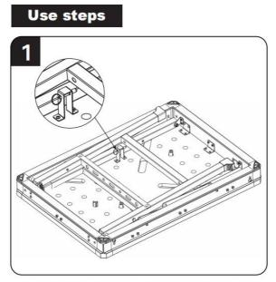
Before using, check that the table is horizontal to use as a work bench, pull out the lock pin to open the leg.
