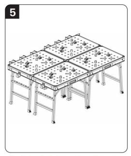
If desired, multiple units can be locked together side by side or end to end with the enclosed joiners.
