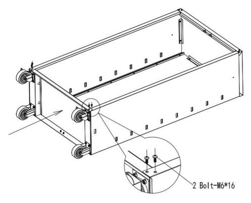
**STEP 6** Flip the body over  $90^{\circ}$ , Install the four bolts-M6\*16(2) on the back as shown.
