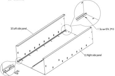
Before assembling the side panels, remove the two U-shaped protection slots at the bottom of the side panels
