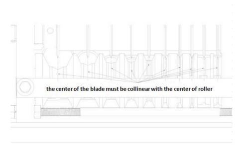
3. According to the thickness of the wire, adjust the height of the blade through the screw above the machine so that the blade can cut the wire skin without damaging the copper core.
