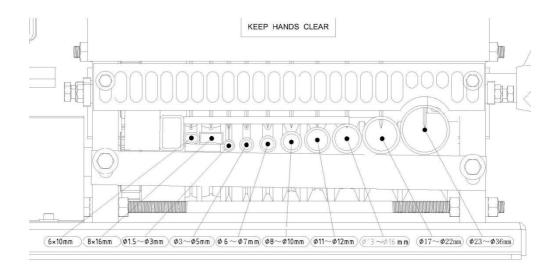
2. During wire stripping, the center of the blade must be collinear with the center of the roller.
