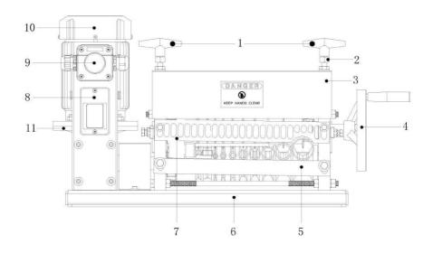
1:M12 Plastic screw 2:Nut for regulating blade up and down
