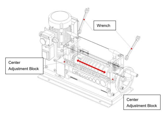
Adjusting the center adjustment block to adjust the blade shaft to the left or right by the wrench.
