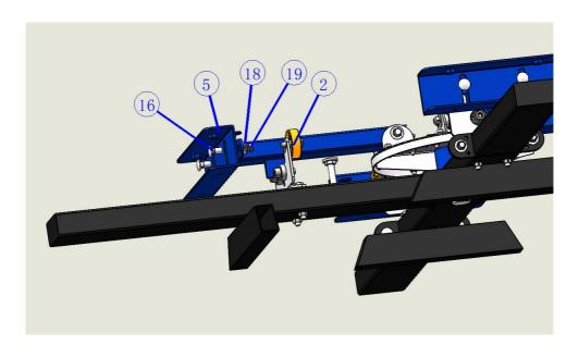
6.Lock the five-star handle(19)into the screen clamp(5)with a depth of 20mm, cover the tabletting(20),and then use a cross screwdriver(2) to lock the tabletting(20) on the five-star handle(19)with a cross countersunk screw M4X8(9) from the small hole at the lower end of the screen clamp(5)
