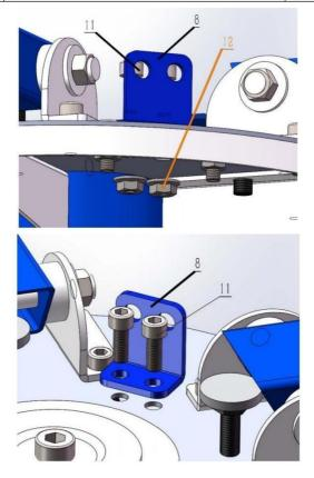
8.Hang the spring(23)on the screen clamp(5),hang the hooked end of the hook(22) on the spring hook plate(8),hook the looped end of hook(22)with the spring(23), and then level the arm support
