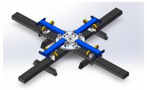
5.Take the screen clamp(5)and stick it to the printing arm(2),insert it into the printing arm(2)hole from the screen clamp(5) with square neck bolt M10X20(16), cover the other end with gasket M10 (17),then lock the outer hexagon nut M10(18), and then lock it with wrench 14-17(—)
