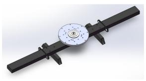
2.Take out the long table support bar (25), put it on the base (1), and lock it with square neck bolt square (17), gasket M10 (18) and external hexagon nut M10 (19). Locking tool wrench 17-17 (I)
