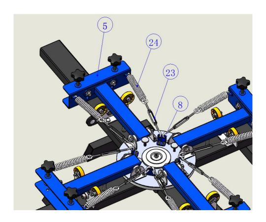
9.Lock the socket head cap screw(13)on the base disc(as shown in the figure),and stick the felt pad(21) to the head end of the socket head cap screw(13). Use tool wrench 14-17(I)
