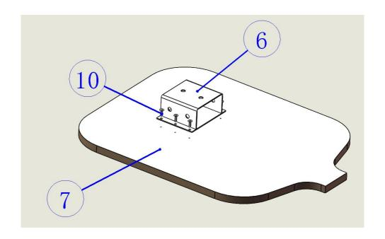
11.Insert the metal bracket(6)in the metal bracket of the wooden platform plate assembled in step 8 into the table support bar(3),and then insert the socket head screw M10X30(14)into the tooth hole of the metal bracket(6),and then use the socket head wrench M10(five)to lock the socket head screw M10X25(14)
