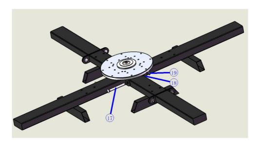
3.Put the positioning seat(4)on the square tube of the base(1),thread it from top to bottom with the external hexagon screw M8X55,and lock the other end with the external hexagon nut M8. Put the outer hexagon screw M10X55(15) onto the outer hexagon nut M10(18)and thread the screw head 40 mm from the base square tube from top to bottom, then lock the outer hexagon nut M10 (18)onto the base square tube in reverse.
