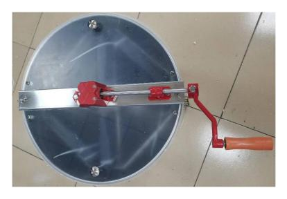
**Step 6:** Rotating honey extractor. Hold the handle with your hand and shake it in the same direction to rotate the inner frame.
