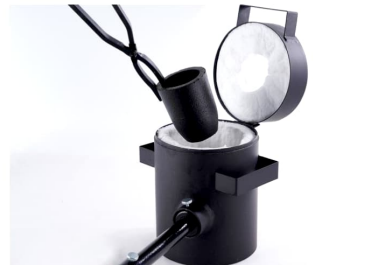
8. Put the crucible in the furnace, light the paper, put the paper in the crucible, open the propane tank.
