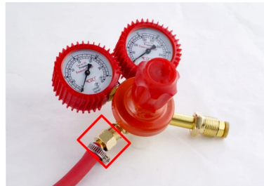
6. Connect the red trachea to the brass, tighten the screws.
