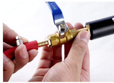
2. Connect the red trachea to the brass, tighten the screws.
