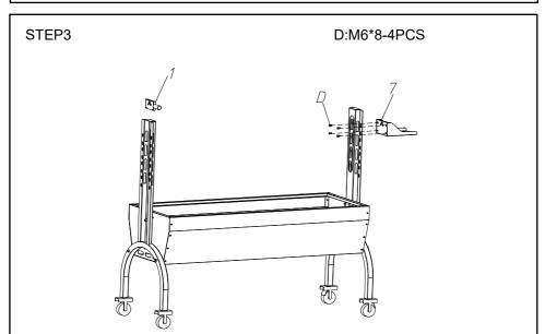
The motor support plate is aligned with the support foot hole position, adjusted to the appropriate height, and fixed with M6\*8 hexagon screws. And put the barbecue fork bracket in the corresponding position of the other supporting foot.
