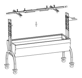
Put the food and barbecue fork together on the motor support plate and spit bracket.
