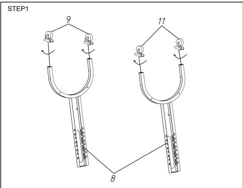
Install four casters on the support foot, rotate and tighten them in the direction of the arrow, and install casters 2 (with brake) on the same support foot.
