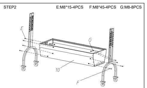
Fix the support foot and grill body with M8\*45, M8\*15 hexagon screws and M8 flange nuts .
