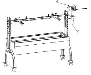
Place the motor on the motor support plate and lock it with M6\*8 hexagon screws. The installation is complete. Put charcoal on the charcoal tray, ignition, can roast sheep and other large pieces of food.
