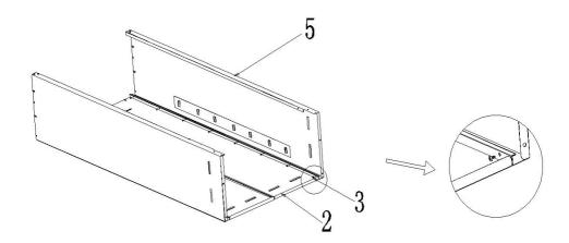
Assemble the kickplate(6) on the inside between left side panel(4) and right side panel(5), aligns holes to two lateral plates, and secure them with 4 M6\*15 bolts.
