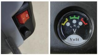
A. Turn on the switch. ("1" means to turn on the power, and "0" means to turn off the power)  $% \left( \left( 1-\frac{1}{2}\right) \right) =0$
