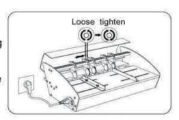
adjust the right and left postioning/ according to the paper size, the scale only for reference, you can fine adjusting the specific direction.
