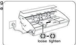
5. put in suitable paper, adjust the creasing pressure and feeding pressure. Different paper with different creasing pressure. You can adjust the right and left press wheel, usually the left
