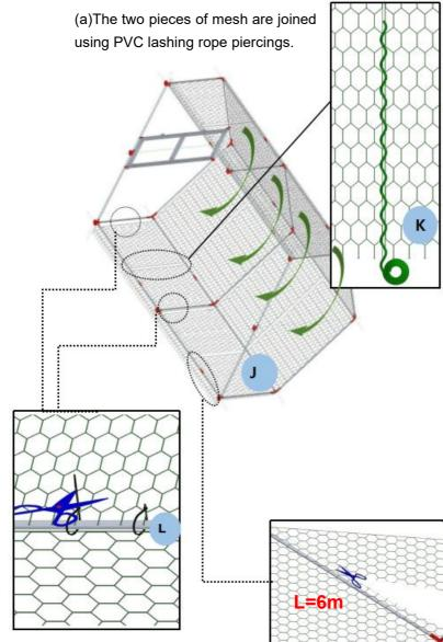
(c)Secure the mesh to the frame with cable ties.
