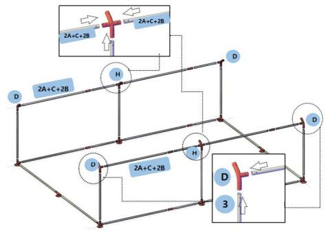
Step5: Install the top surface according to the part number in the figure below.
