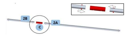
Step2: Install the bottom frame according to the part number in the picture below.
