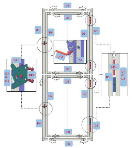
Step7: Attach the door to the frame.
