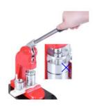
Place pinned back (zigzag side of pin showing) in right hand die. Press down the handle to complete assembly. There must be no gap in the top die when you press down the handle.
