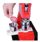
Place metal badge top (rim down) in left hand die in the circular slot. Cover with cut out print (printed side up) and one plastic film.
