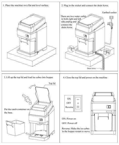
2. Find a flat location for the appliance where it's protected from direct sunlight and other heat sources (i.e., stove, furnace, radiator). Place the appliance on a
