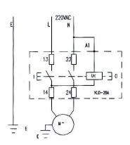
KLD: Switch M: Motor FA: Thermo-protection of the engine
