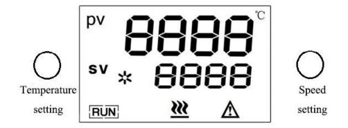
PV means the temperature, when there is no external sensor, it means the furnace plate temperature, when the external sensor is connected, it means the external sensor temperature.
