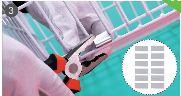
3. Fix with 12 metal pieces (J). Note: Need to use pincer pliers and gloves to prevent injuries
