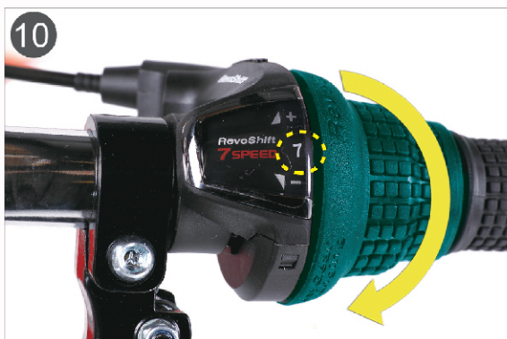
10. Special Note: When installing the transmission, the front shifter should be adjusted to the 7th speed.
