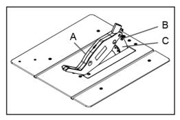
Do not screw in the bolt(B) too tightly; the saw blade guard(A) must move freely.
