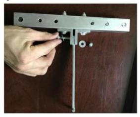
4.Assemble carriage bolts (No11), nuts and washer (No.12) through cross bar (No.2) leave loose. Head of carriage bolt must be as shown.
