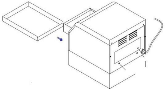
2.5. Back tray installation: Insert the back tray to the hook of the back tray following the arrowhead (picture three).
