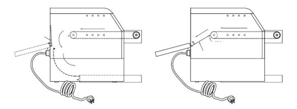
2.4. Down tray installation: Insert the down tray to the hook of the down tray from the back of the appliance following the arrowhead (picture two).
