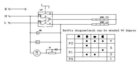
HL1-----Power indicator lamp ∞-----Fan EHI, EH2-----Electric heating elements R-----Speed regulator M-----Motor QS.-----Switch
