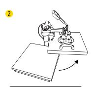
Rotate the heat transfer board to the side.
