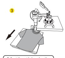
Pull out the mat below, place the clothes flat on the mat, and place the pattern on the clothes.
