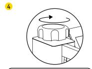
Turn this adjustment switch to adjust the pressure.
