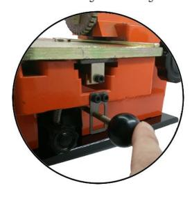
5, Close the clutch and lock the work table and lock the carriage.
