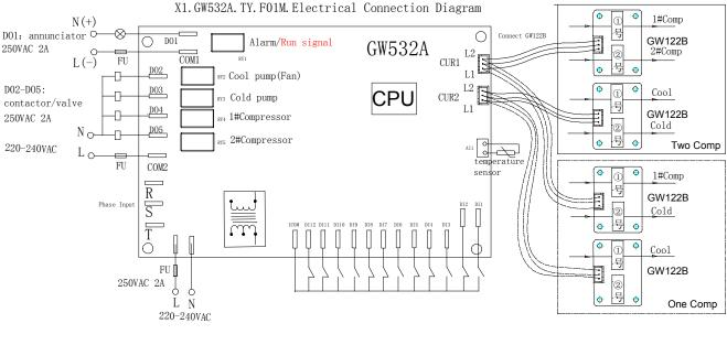
DI1:Cool overload/Antifreezing switch DI2:Remote switch DI3:Cold Pump overload DI4:Cold Water flow switch DI5:Water level switch/Vent1 temperature DI6:1#Compressor overload DI7:Low pressure of 1#compressor DI8:High pressure of 1#compressor DI9:Cool flow switch/Vent2 temprature/Phase switch DI10:2#Compressor overload DI11:Low pressure of 2#compressor DI12:High pressure of 2#compressor
