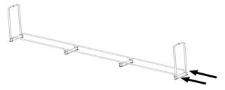
5. After assembly is completed, the L-shaped connection pad is fixed with expansion screws in the middle to increase the stability of the rack. The holes on the side of the connection pad are pre-drilled and can be fixed freely as required. As the picture shows:
