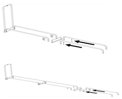
4. Assemble another side frame with the completed part of step 3, then fasten with 4pcs M8\*60m screws and nuts. As the picture shows:
