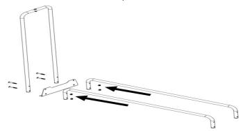
3. Connect 2pcs L-shaped frame and 4pcs of U-shaped connectors tube to the already assembled part and fasten with 4pcs M8\*60m screws and nuts. As the picture shows:
