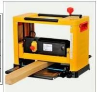
At first, the user needs a ruler to measure the thickness of the wood to be planed. Then observe the depth label (H) to adjust the depth label to the thickness of the planer required by the user.
