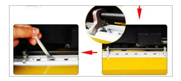
**Warning!** Check that total 18 screws are tightened. Turn the blade holder by hand to check that it rotates easily and smoothly.
