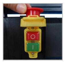
This planer is equipped with an electromagnetic switch.
