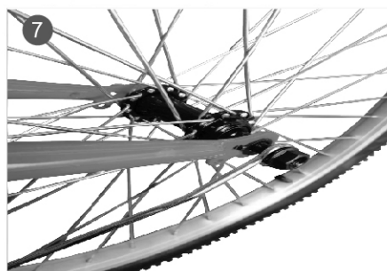
7. Cover the front axle plug.
