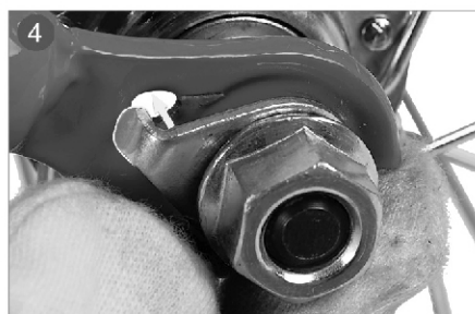
4. Special Note: There is a hook on the washer. Let it hook into the hole in the front fork for better fixing.
