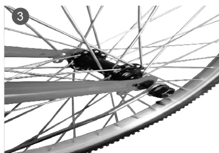
3. The hook is on the inner mud board and the middle nut is on the outside
