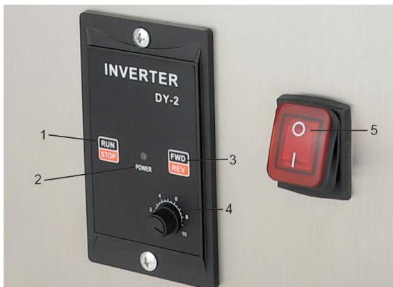
Controller 1. The Stop/Start button. 2. Indicator light. 3. Rotate forward and backward buttons. 4. Speed regulating potentiometer knob adjustable speed range 0-2980 RPM. 5. Machine switch
