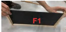
Step 2: Connect with nails at a/b/c/d 4 positions.
