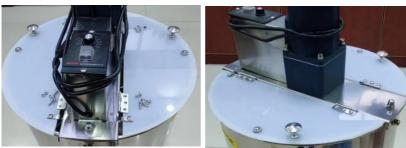
Assemble the two lids with screws.
