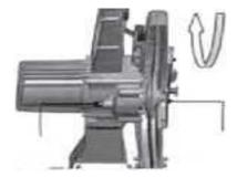
10.3 When installing the saw blade, make sure that the arrow on the blade points in the same direction as the arrow on the blade cover. When installing the saw blade, make sure that the inner hole of the saw blade is flat on the output shaft.
