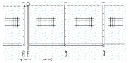
3.Drill hole around the entire pool with 17mm drilling guide. All holes should be drilled to a depth of 4", and at a direct 90° angle to the deck.
