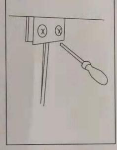
Step 2: Connect the pairs of glass panels at the bottom using the other two linear connectors. Two cylinder feet can be applied about 1 inch away from each side of the bottom linear connector.
