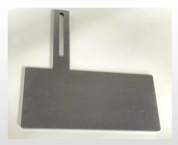
Solid steel tool rest, 3/8" thick unfinished steel. This rest bolts directly onto a 1.5"x1.5" main tooling arm, or to an extra tooling arm in the bottom slot of the grinder. The slot allows it to be moved closer to or further away from the belt. We leave the surface unfinished: sand it smooth or drill & tap it easily for your fixtures. Also easy to weld angles or holding plates onto.
