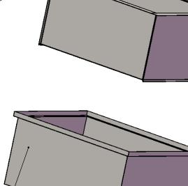
The box body is designed as a double layer with insulation cotton in the middle layer
