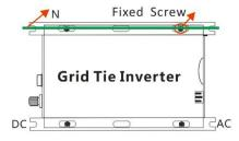
3. Properly connect the positive and negative of solar panel and Smart Microinverter,
