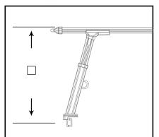
Loosen the screw on the post, adjust to the desired height, and observe the position of
