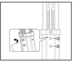
Loosen ①② screws properly, do not loosen all screws.
