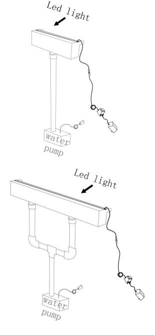
**Note:** This is just a brief installation, customers should prepare different necessary accessories before installment, for example, a suitable water pump and water pipe.
