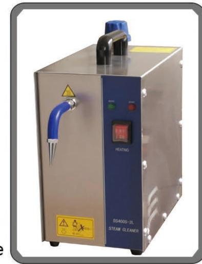
boiler reaches over 3.5 bar, the steam cleaner enters into working state, the temperature of the spraying saturated steam reaches over 135°C, use the high temperature and high pressure of saturated steam to remove the attachments such as oil stain, sewage from the surface of the parts and vaporize them away. At the same time, it can also clean small gaps and holes, peel off and remove oil stains and residues to achieve requirements for high efficiency, water saving, clean and dry.
