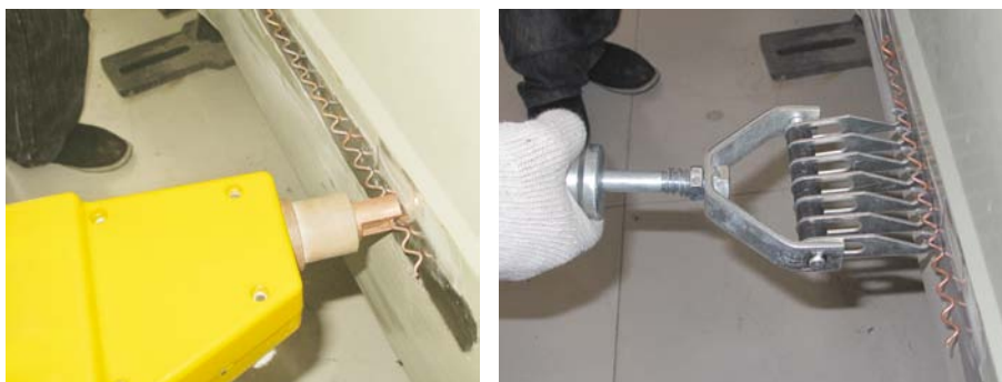
Wavy-wires welding and pulling
